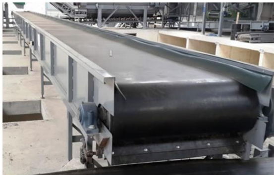
Heavy Duty Manual Sorting Conveyor showing the lateral edges to insure proper sealing of the conveyor and minimize waste or leachate leakage to the center of the conveyor – Nabatiyeh – Lebanon
