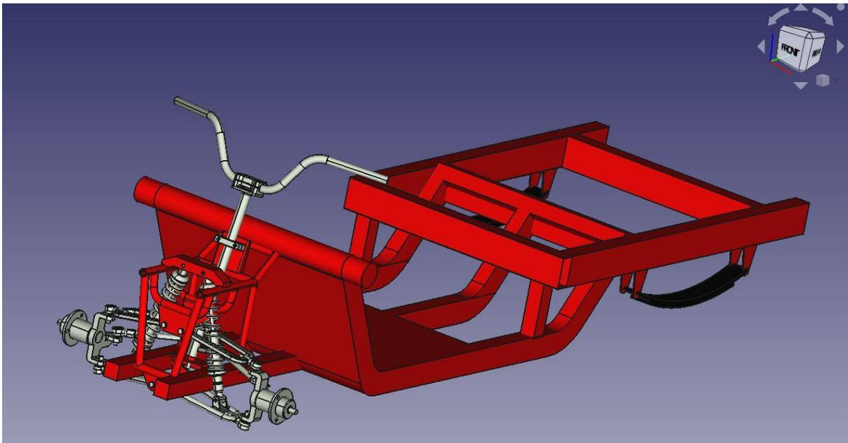
**3.2.1.1 FreeCAD design 7-11-2023 new chassis with front suspension:**
