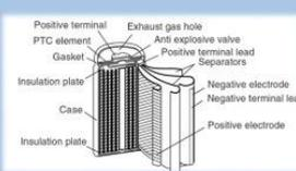
Lithium-ion cells - The lithium-ion battery is surrounded by a metal casing, and this metal casing is necessary to protect battery contents. The cover contains special safety when the temperature rises. The battery pressure increases beyond the permissible limit.
