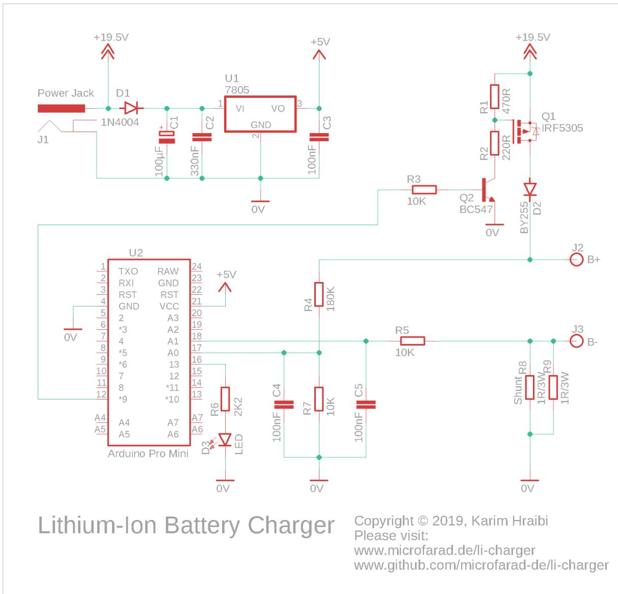
**Figure 3: Li-Ion charger circuit diagram**
