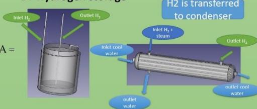
When Hydrogen gas exits from the condenser, it is pumped to the compressor at 30 bar then it storage in hydrogen tank
