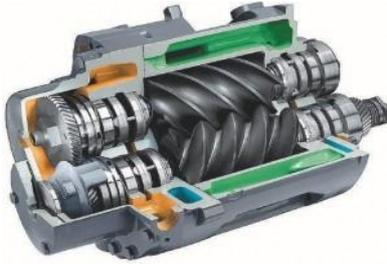
Twin screw shaped meshing rotors are mounted in a figure of eight shaped housing, which has suction and discharge ports at either end. As the rotors turn they form a space that traps gas, the space travels down the length of the housing, and because of the profile of the screws, is compressed as it goes. Due to no lubricant in the compression space, timing gears are employed to ensure that the two rotors do not touch.
