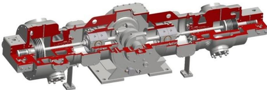
Similar to an automotive combustion engine, except passive non return valves replace actuated valves. A piston travels up and down inside a cylinder, and is connected to a crank shaft by a connecting rod. On the intake stroke, the discharge valves are forced shut, and gas is therefore sucked into the cylinder.
