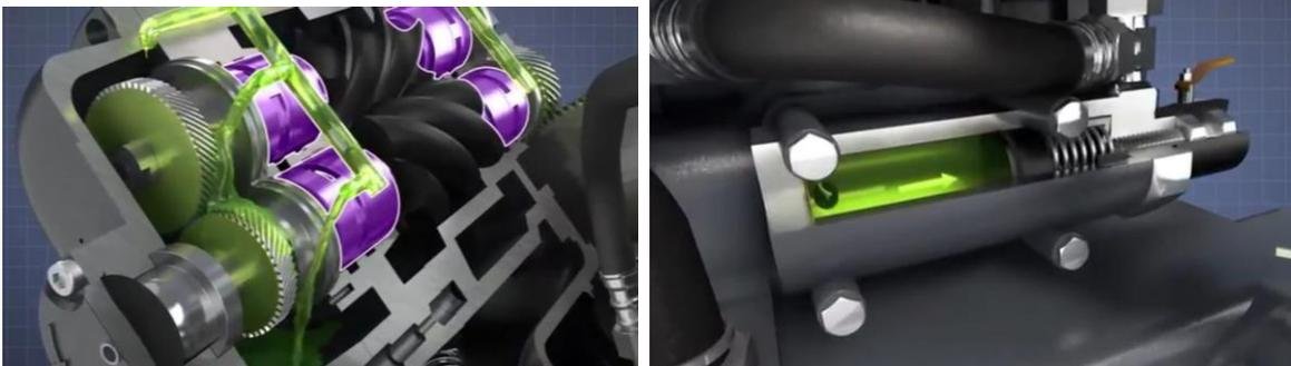
Oil is topped up via a fillip pipe at the front to the air end. The compression process is kept cool by a constant flow of water passing through channels that surround the air end rotors. Heat transfers to the water which is then pumped through an external cooler before returning to the air end.
