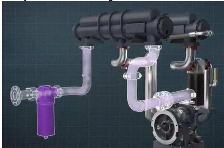
The air then passes through a final second stage air or water cooling process to ensure the delivery air is at the right temperature. Then after a final journey through a moisture separator, the air is ready to exit the compressor at the delivery port.
