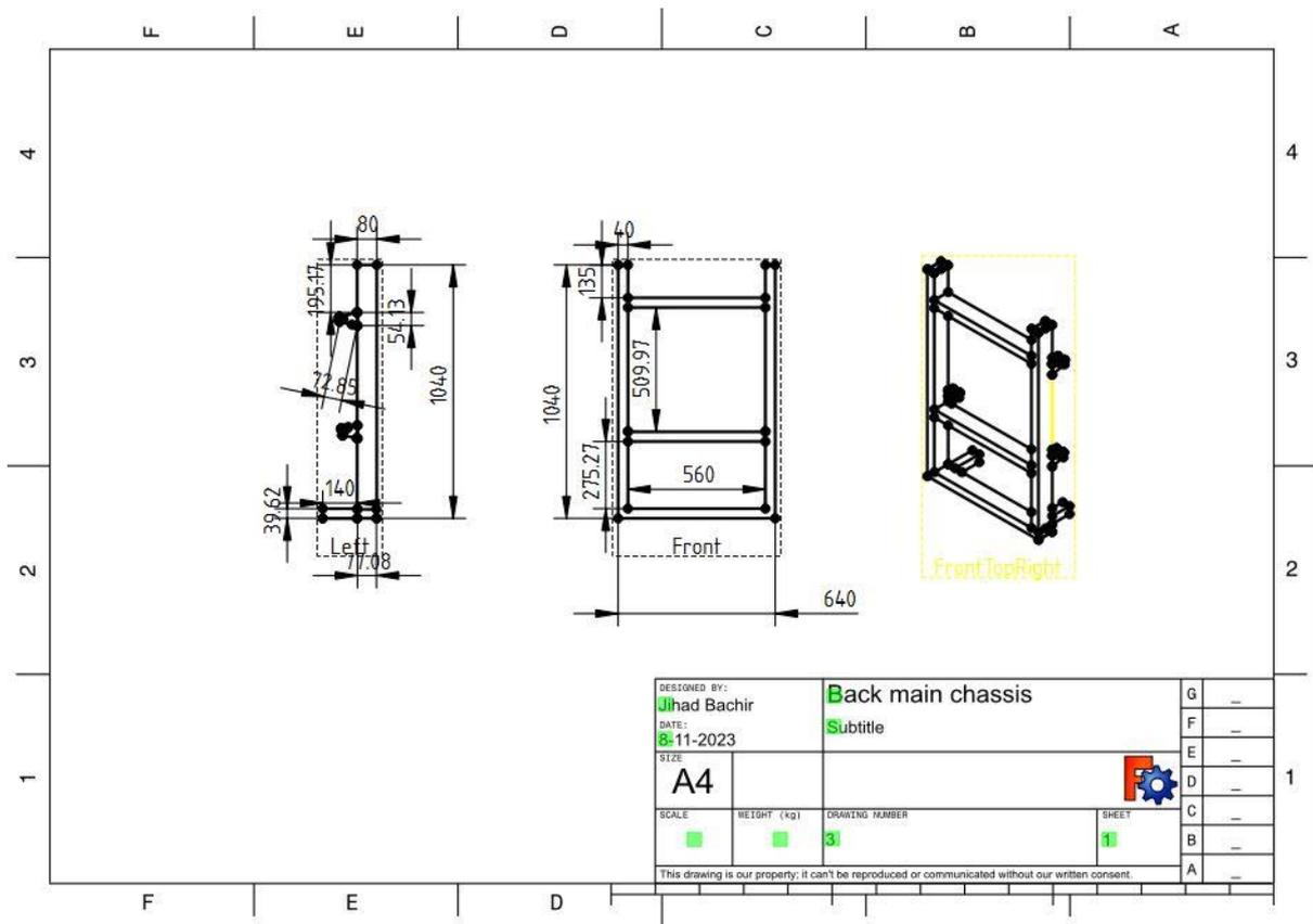
[2d and 3d drawing of the back part of the main chassis :](#)
