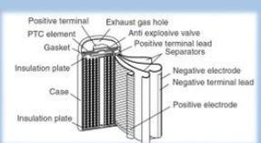
Lithium-ion cells - The lithium-ion battery is surrounded by a metal casing, and this metal casing is necessary to protect battery contents. The cover contains special safety when the temperature rises. The battery pressure increases beyond the permissible limit.
