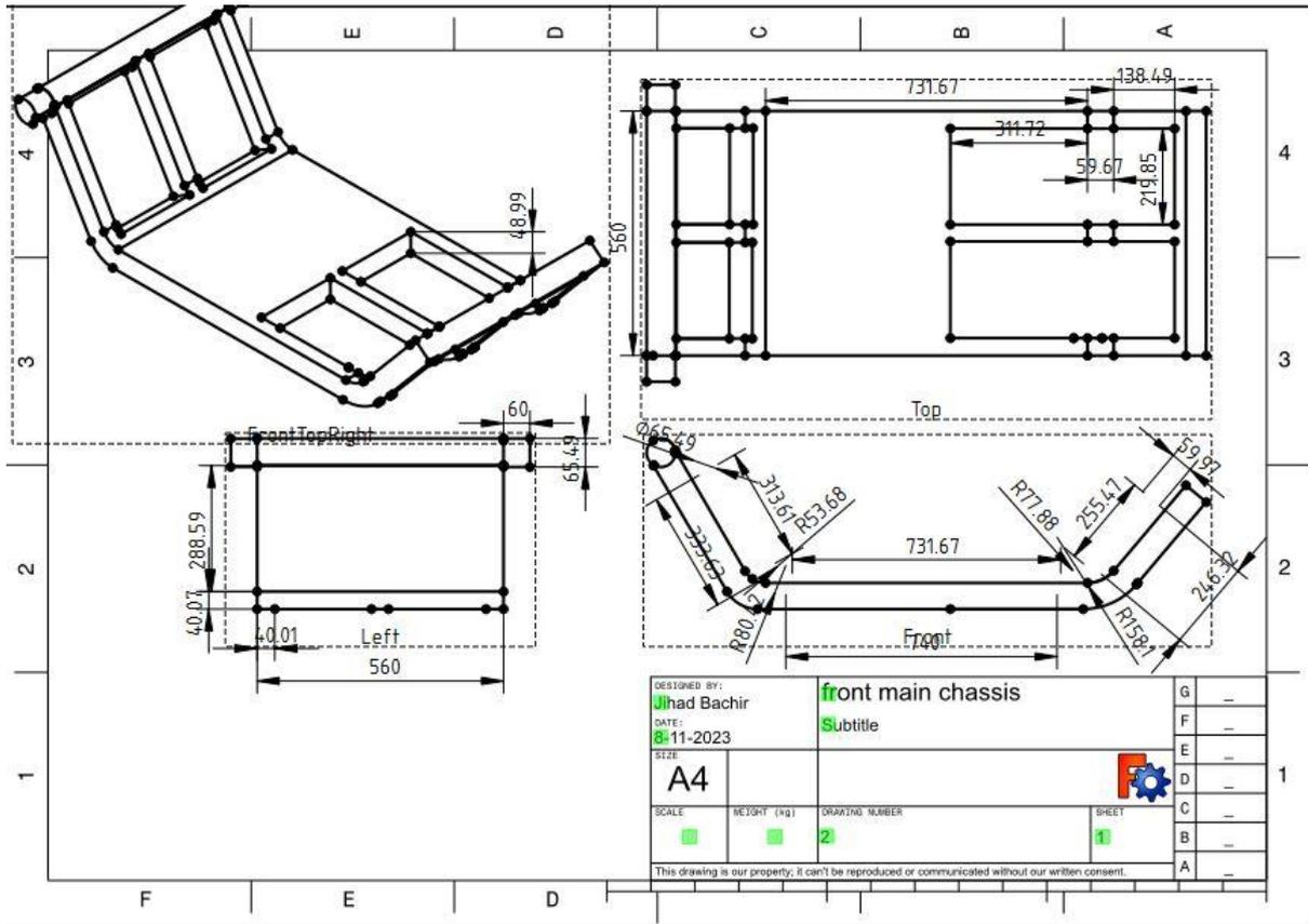
[2D and 3D drawing and techdraw for the front main chassis design :](#)
