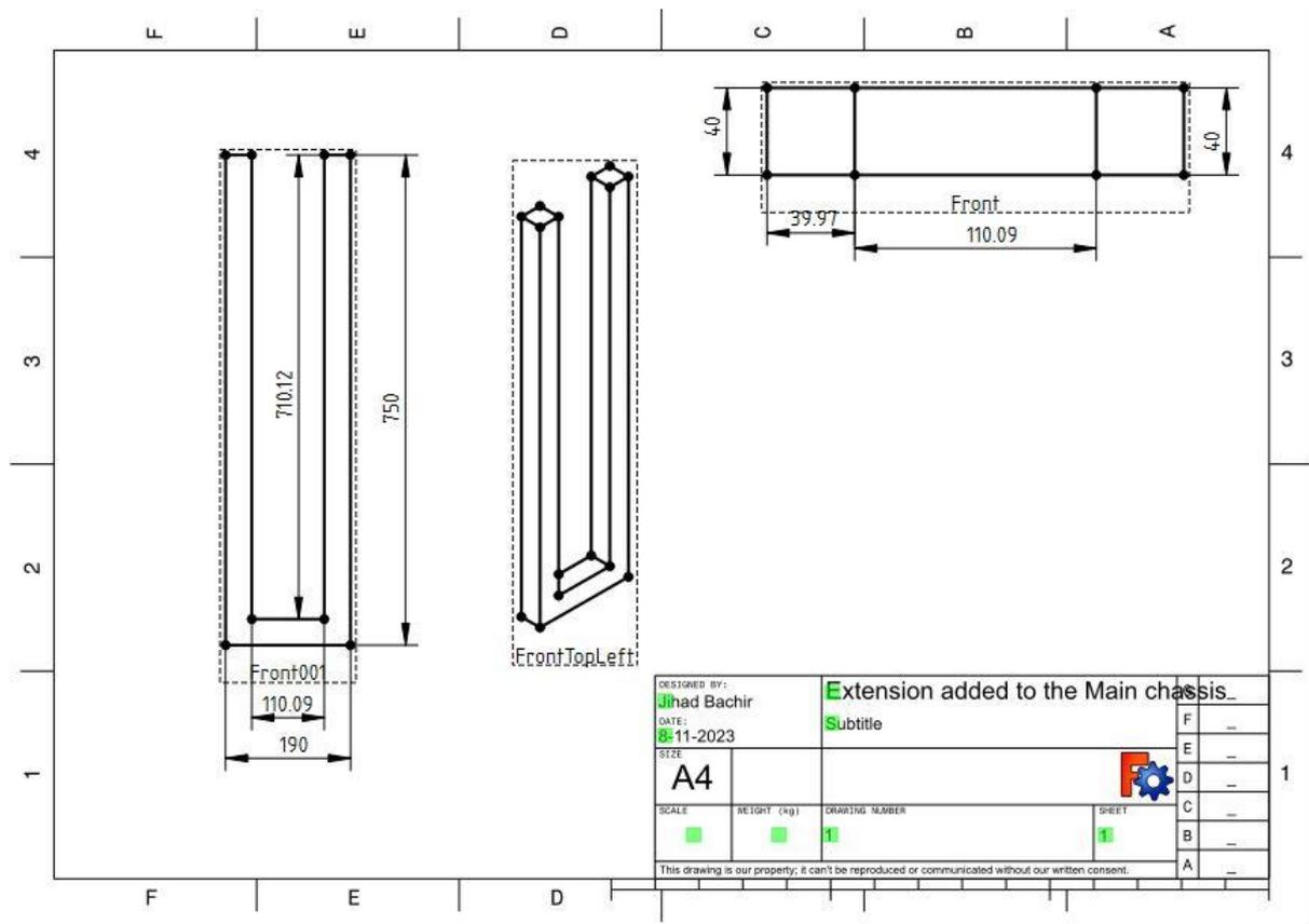
[FreeCAD 2d and 3d drawing of the extension link between front suspension and main chassis :](#)
