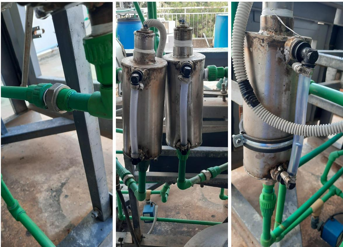
Also, we couldn't see air bubbles in the oxygen water receiver, but we saw them a little in the hydrogen water receiver.
