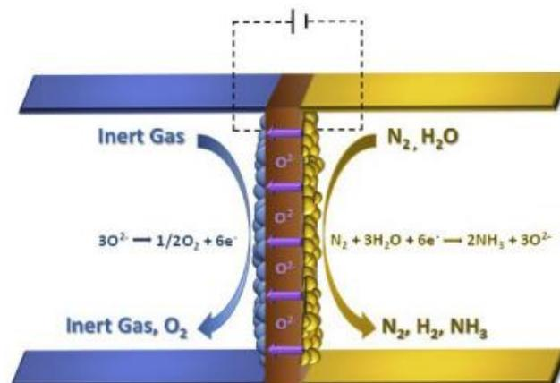
**Fig. 3.** A schematic of the SSAS process where an oxygen ion (O<sup>2-</sup>) conductor is employed as the electrolyte.
