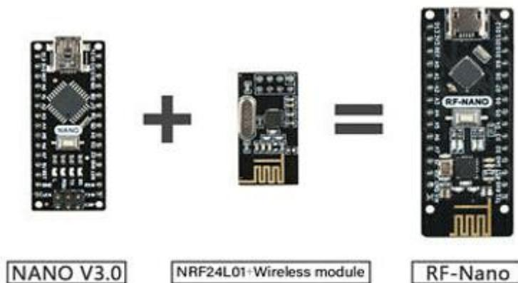
Figure 10. Arduino Nano RF
