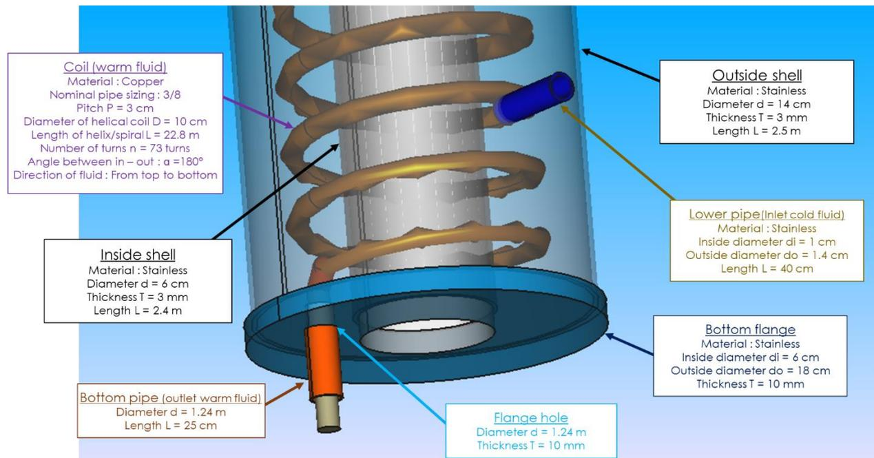
**5) Heat exchanger - Thermal calculation****a) Average temperature LMTD  $\Delta t_m = ?$**
