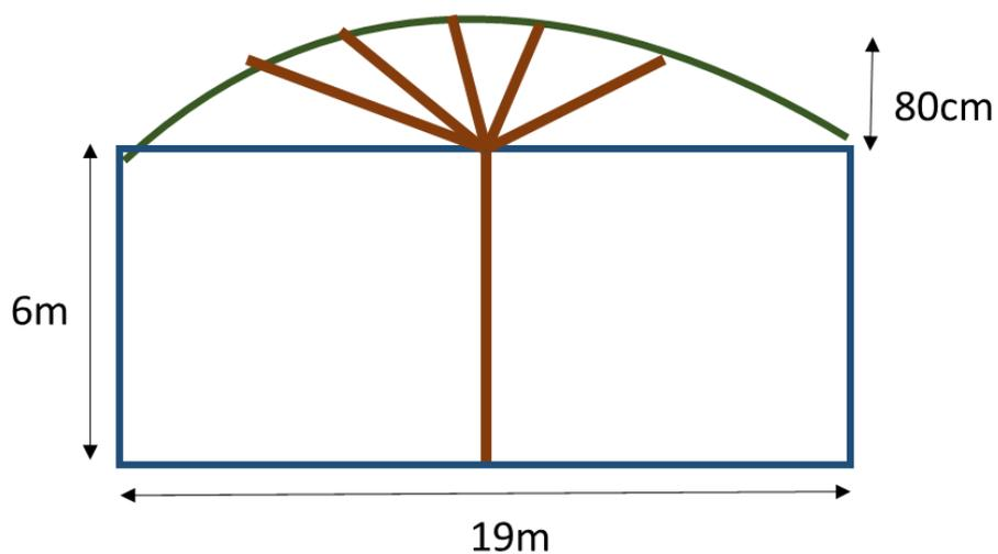
A digester diameter of 19 m allows a hydraulic retention time of 44.1 days
