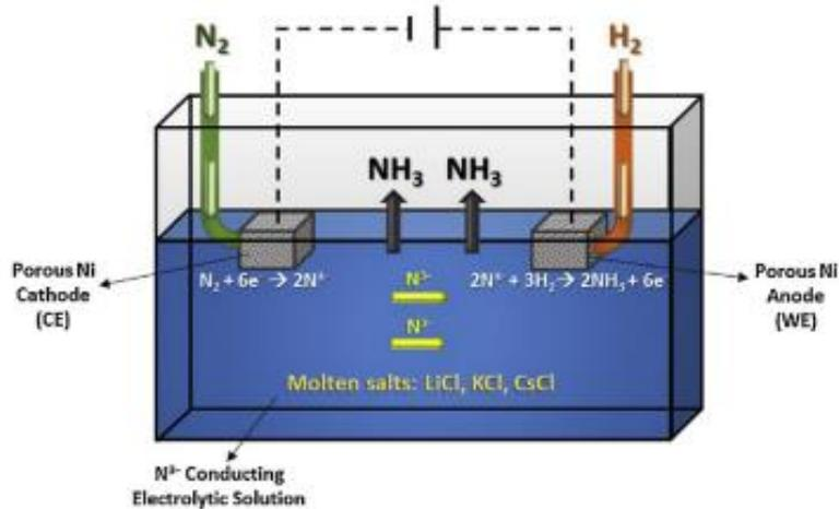
Fig. 4. Apparatus used by Murakami et al. [55]. The electrolyte was a N<sup>3-</sup> conducting molten salt mixture (57.5LiCl, 13.3KCl, 29.2CsCl mol%) and nitrogen was reduced on a porous Ni cathode.
