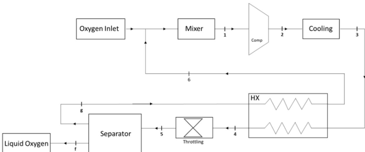
In our prototype, we decided to dispense with the heat exchanger in order to avoid expensive materials and manufacturing costs. However, through the theoretical study, it was found that we will face a problem in reaching the required liquefaction temperature, in addition to the compressor failure due to the low gas temperature at the compressor inlet.
