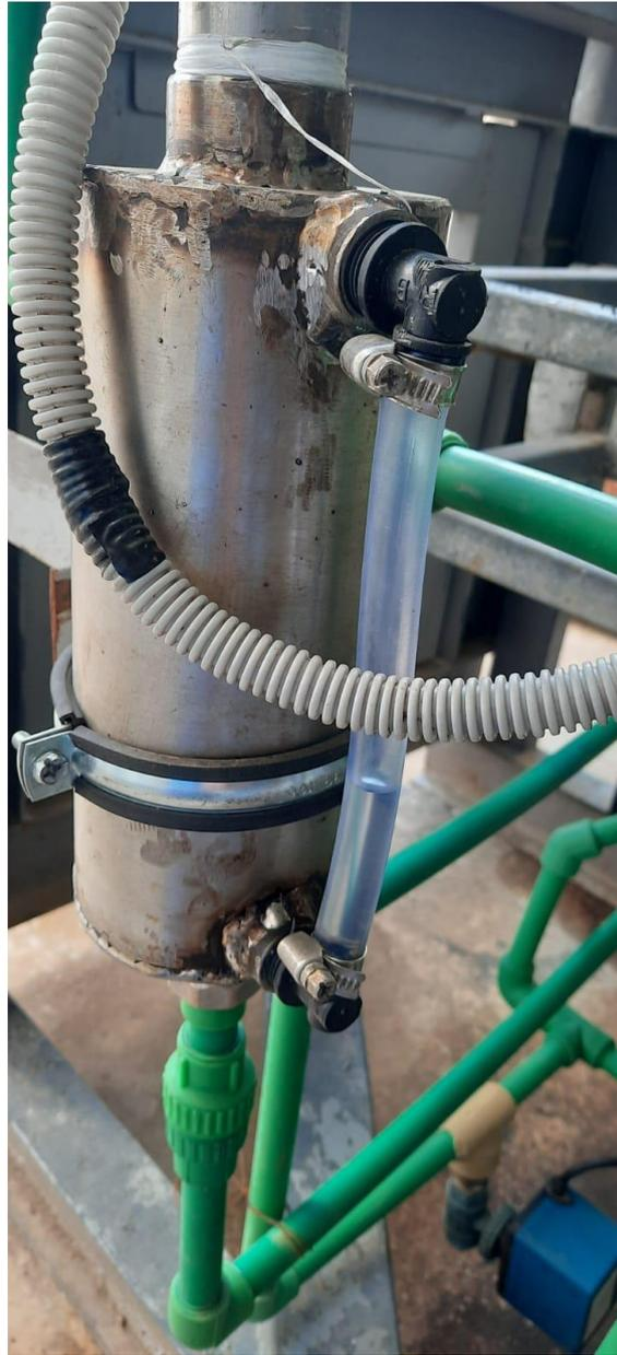
Also, we couldn't see air bubbles in the oxygen water receiver, but we saw them a little in the hydrogen water receiver.
