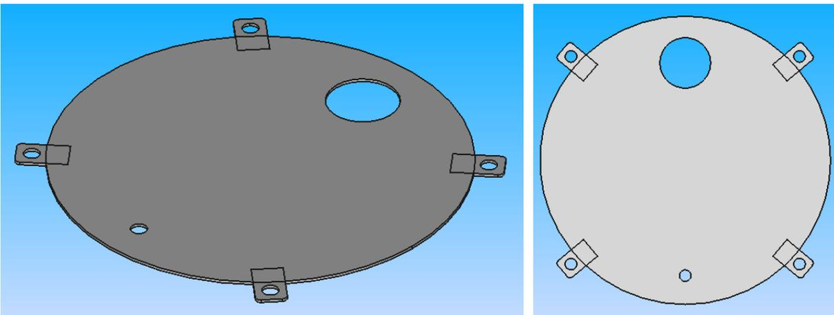
**m) Electrolysis step 4 & 5 \_ End plate 2 (Outlet solution)**
