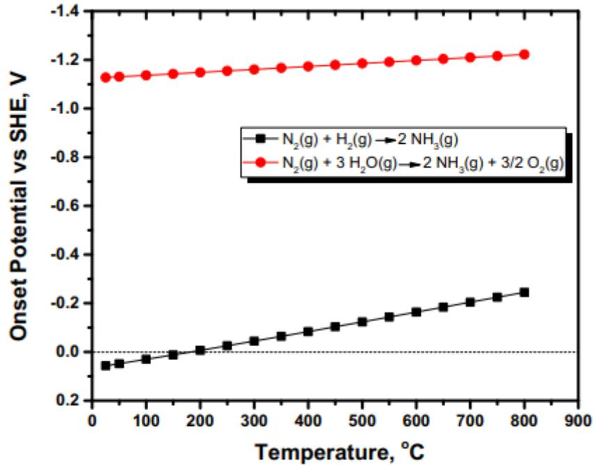
**Fig. 8.** Dependence of the equilibrium potential (calculated from equation (19)) on the operating temperature for the electrochemical production of ammonia from hydrogen (squares) and steam (circles).
