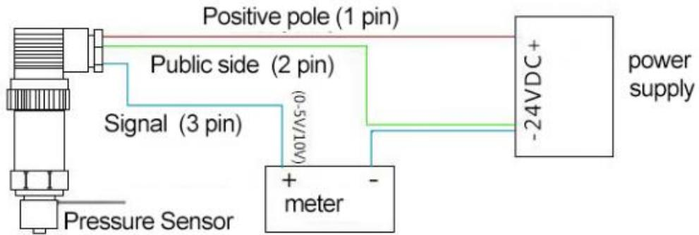
Red line: 24VDC Blue line: voltage output + green line: power supply -
