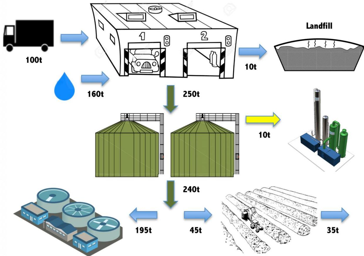
For example, 100 tons of solid municipal residential source separated organics (SSO) arrives at the biogas plant using wet digestion (complete mix). This feedstock needs to be pretreated to remove potential contaminants (plastics, metal, sands, etc.). Approximately 10 tons will be removed as contaminants and will probably be landfilled.
