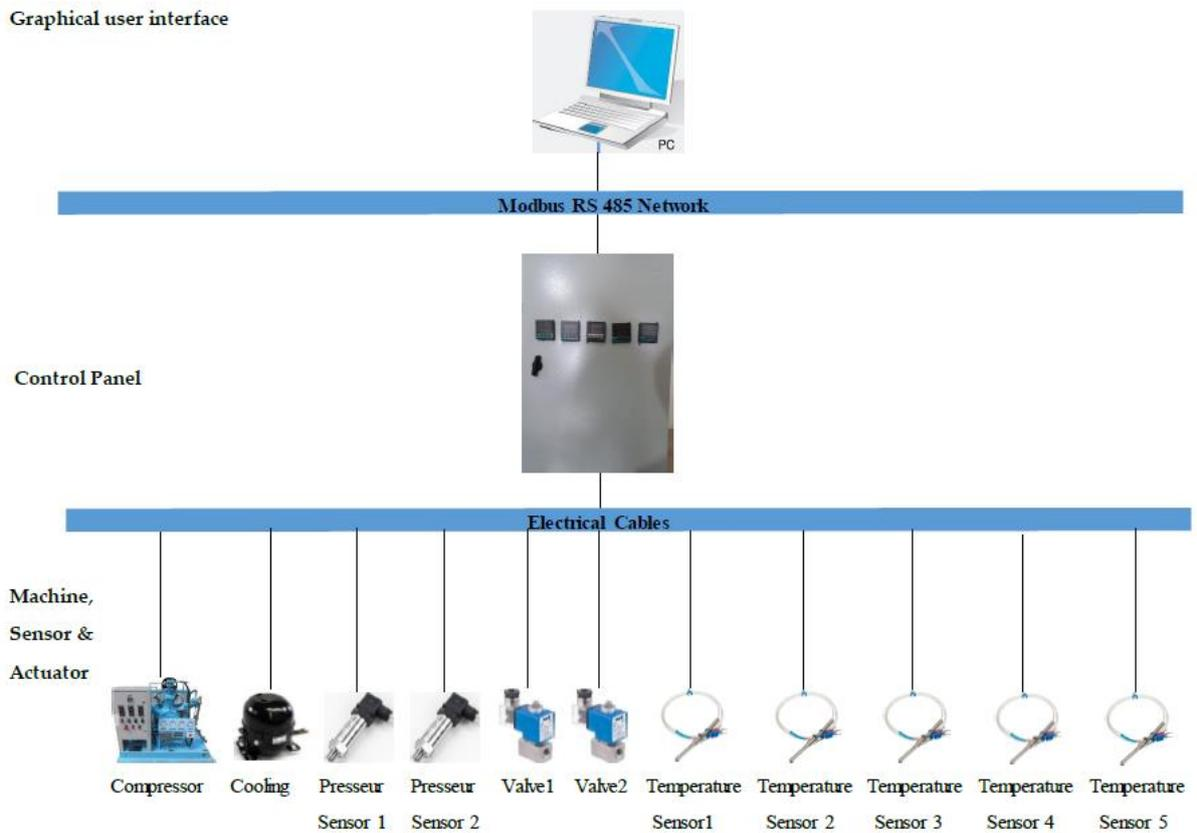
The process control system is the same for the LOX system with/without a heat exchanger (HX) (Version 2021)
