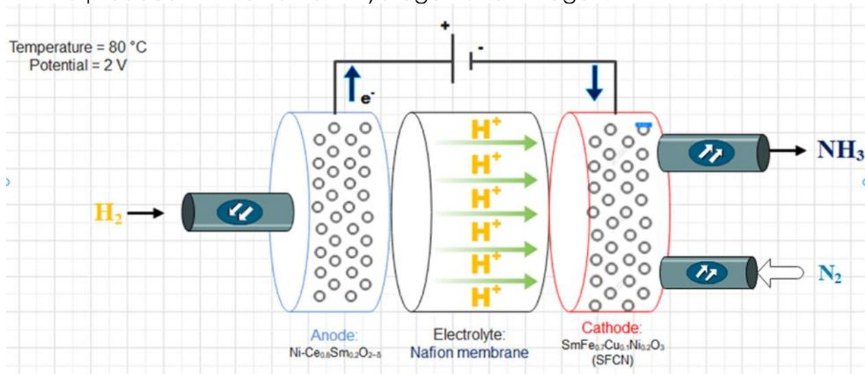
Electrochemical methods of ammonia synthesis have been most widely studied. It is recognized that Nafion is the best polymer proton exchange membrane.
