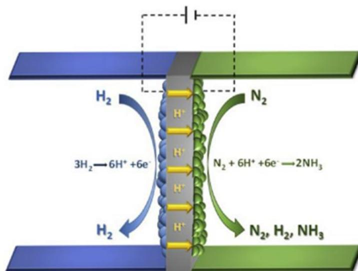
**Fig. 1.** Schematic diagram of the solid state ammonia synthesis (SSAS) process in a double chamber proton conducting reactor cell.
