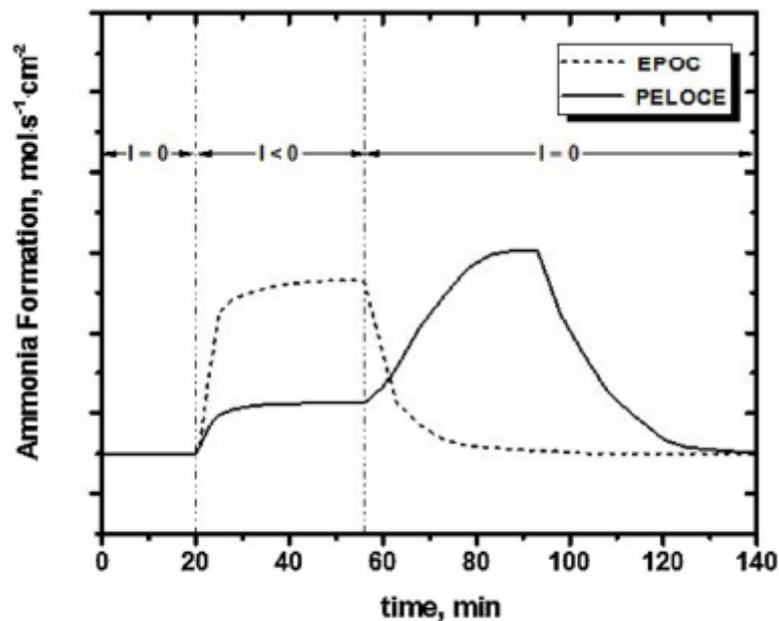
**Fig. 10.** Ammonia formation rate transients during typical EPOC (dotted line) and PELOCE (continuous line) experiments [89].
